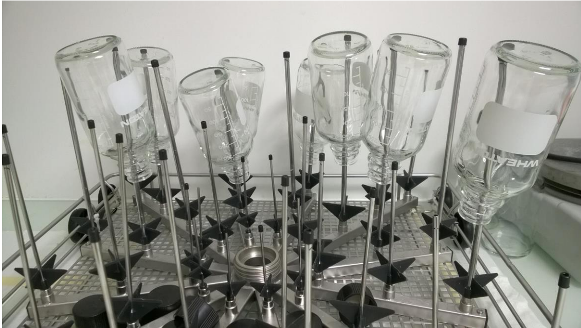
Figure 1 - Dry the bottles upside down raised by a support
