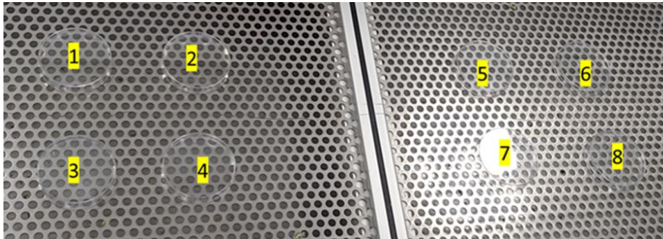
Figure 10: Layout of petri dishes within the Horizontal Track Sprayer
