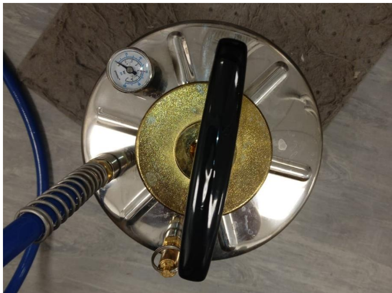
Figure 7: Inlet pipe inserted directly to the top of compression sprayer.
