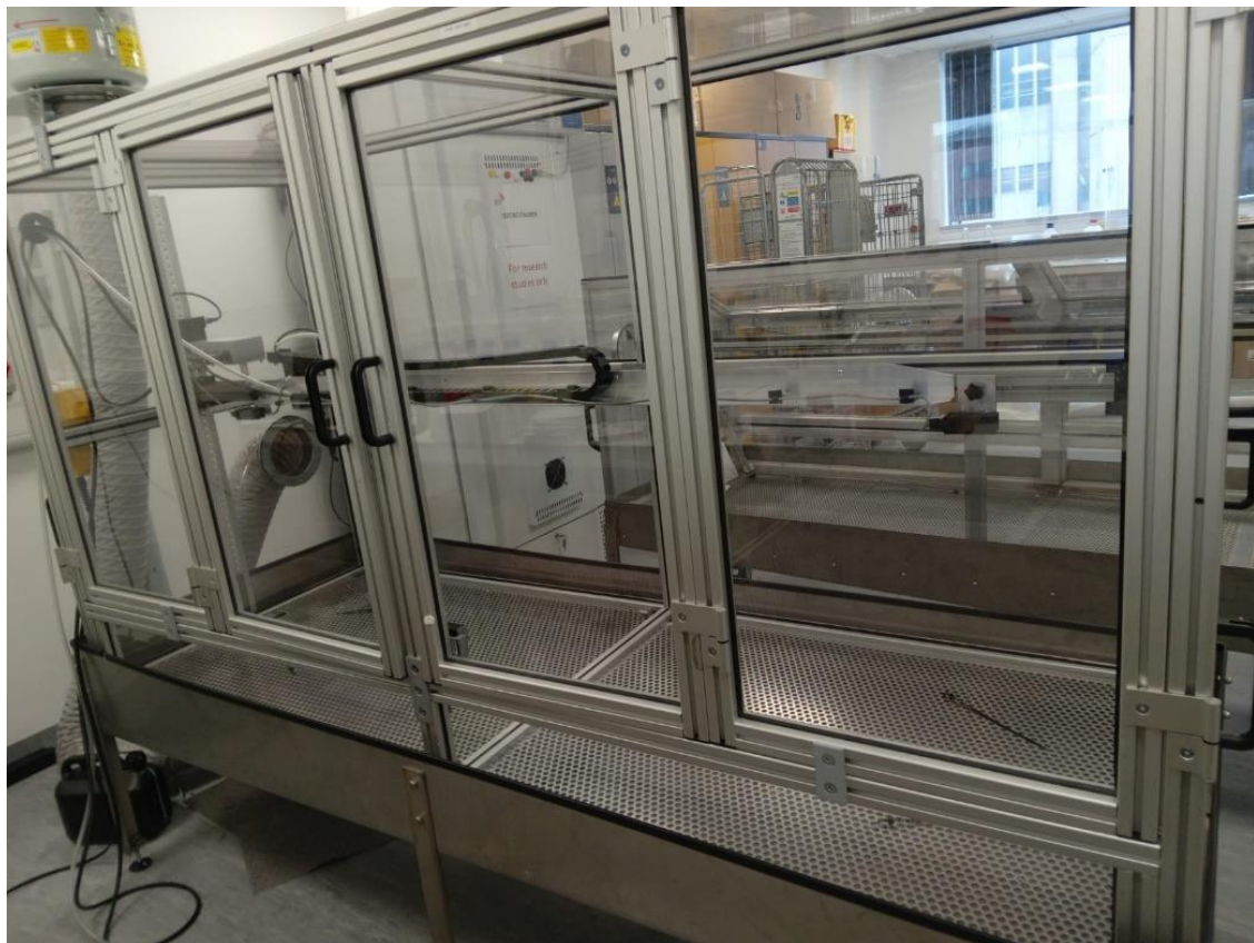
Figure 1. Set up of the track sprayer in the enclosed Perspex chamber.
